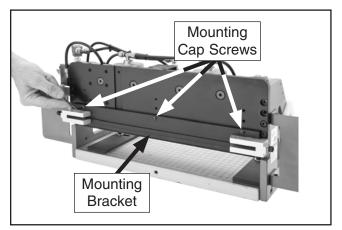
Figure 12. Installing template mounting bracket.
